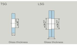
Corner connectors glass / glass (dimensions in mm)
