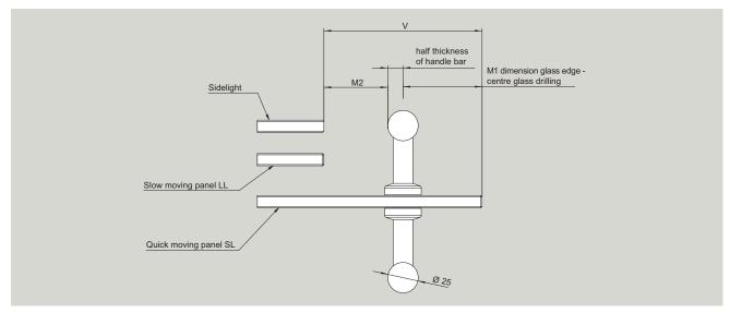
$\mathsf{V}$  = Protrusion of the quick-moving panel (SL) when fitted with a pull handle (see Data Sheet 36-747)
