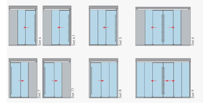
Glass door (8 - 13.5 mm) with glass overpanel and glass side lights (10 - 19 mm) - 2 and 4 panels
