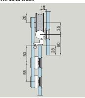
Sliding door with tubular track and clamp fixing
