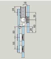
Countersunk bore for countersunk singlepoint fixings
