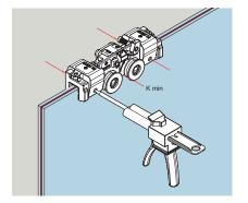
DORMA-GLAS Clamp&Glue technology provides the possibility to keep the advantages and – at the same time – to eliminate the potential issues of laminated safety glass.
