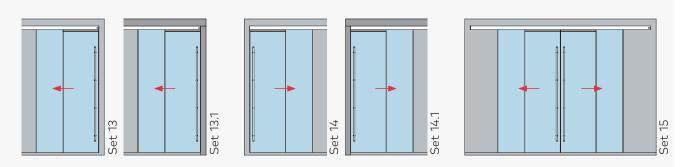
Glass door (8 - 13.5 mm) for the installation at ceiling / with side light (10 - 19 mm) - 2 and 4 panels
