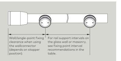
**Caution!** Ensure that the stops/single-point fixings are positioned at locations appropriate to the width of the door.
