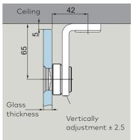
**Note:** Ensure compliance with minimum glass/bore clearances as per glass manufacturer recommendations. Glass preparation with a tolerance of max. ± 0.3 mm is recommended.
